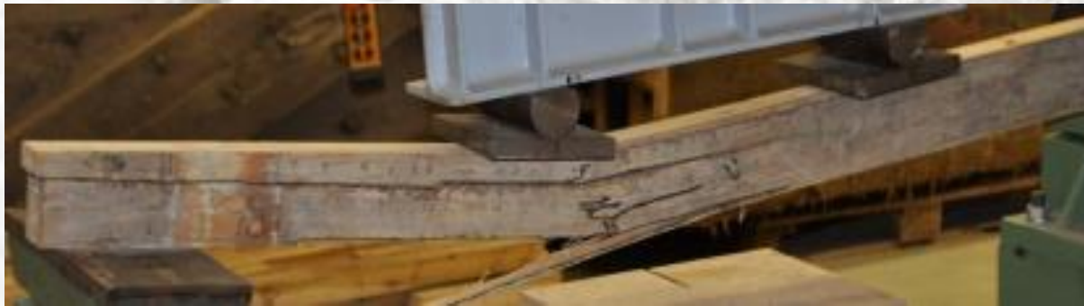
Additional shear fracture on glulam timber
