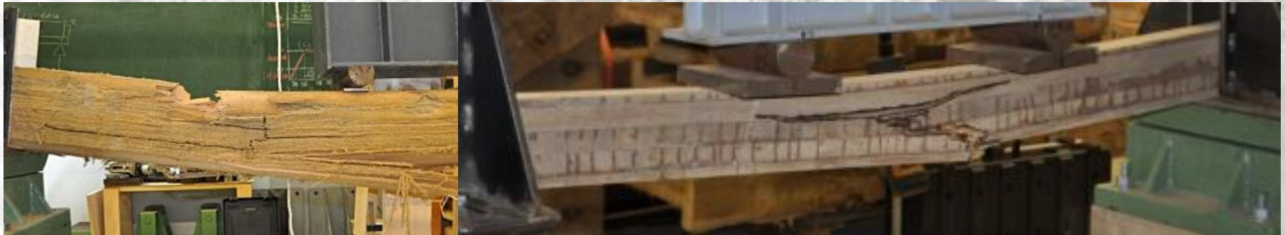
Bending tensile/ compressive on solid and glulam timber
